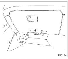
1. Remove the 2 lower glove box hinge pins. Remove the glove box from the opening and let it hang by the cord.
