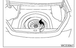
Removing the bolt-on wheel cover (if so equipped)
