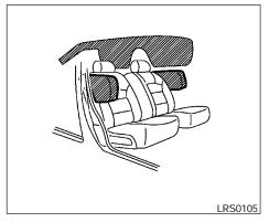
Supplemental side-impact air bag and curtain side-impact air bags system (if so equipped)
