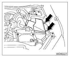
The air cleaner filter should not be cleaned and reused. Replace it according to the maintenance intervals shown in the "NISSAN Service and Maintenance Guide." When replacing the filter, wipe the inside of the air cleaner filter housing and the cover with a damp cloth.
