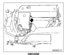
CHECKING ENGINE OIL LEVEL
