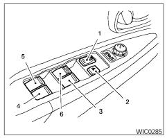
is opened during this period of about 45 seconds, power to the windows is canceled. To open a window, push the switch and hold it down. To close a window, pull the switch up. To stop the opening or closing function at any time, simply release the switch.
