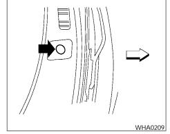
The sunload sensor, located on the top passenger side of the instrument panel, helps the system maintain a constant temperature. Do not put anything on or around this sensor.
