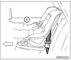
After the child restraint is removed and the seat belt is fully retracted, the automatic locking mode (child restraint mode) is canceled.
