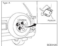
Tightening torque of nuts: 48 to 66 ft-lb (66 to 89 N·m)
