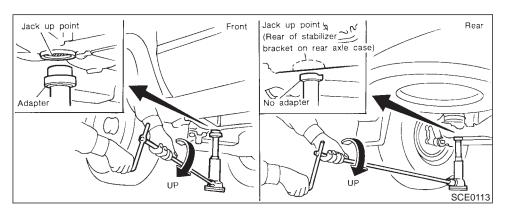
Jacking up the vehicle and removing the damaged tire
