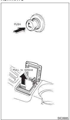
The cigarette lighter operates when the ignition switch is in ACC or ON.
