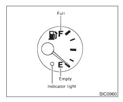
convenient, preferably before the gauge reaches "E". There will be a small reserve of fuel in the tank when the fuel gauge needle reaches "E".
