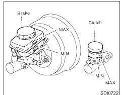
Check the fluid level in the reservoir. If the fluid level is below the MIN. line or the brake warning light comes on, add DOT 3 fluid up to the MAX. line.
