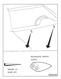
If you wax the surface of the hood, be careful not to let wax get into the washer nozzle. This may cause clogging or improper windshield washer operation. If wax gets into the nozzle, remove it with a needle or small pin.
