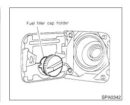
Put the fuel filler cap on the cap holder while refueling.
