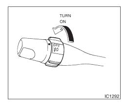
To turn the fog lights on, turn the headlight switch to the  $\underset{\text{$\not =} \ }{\text{$\not =}}$  position, then turn the switch to the  $\underset{\text{$\not =} \ }{\text{$\not =}}$  position. To turn them off, turn the switch to the OFF position.
