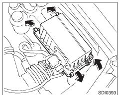
The filter element should not be cleaned and reused as it is given a special treatment. We recommended it be replaced according to the maintenance intervals. See "Periodic maintenance" in the "9. Maintenance" section for maintenance intervals. When replacing the filter, wipe the inside of the air cleaner housing and the cover with a damp cloth.
