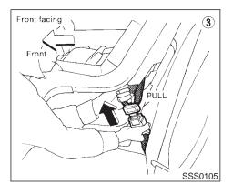
3. Remove all slack in the lap belt for a very tight fit by pulling forcefully on the lap belt adjustment.
