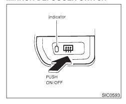
To defog the rear window glass and the outside door mirrors, start the engine and push the switch on. (The indicator light will come on.) Push the switch again to turn the defogger off.
