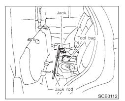
Getting the spare tire and tools Remove jacking tools and spare tire from storage area.
