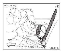
After the child restraint is removed and the seat belt is allowed to wind back into the retractor, the automatic locking mode (child restraint mode) is canceled; the seat belt only locks during a sudden stop or impact.
