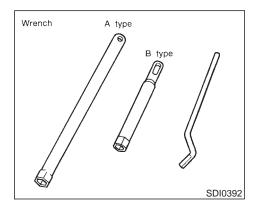
Remove spark plugs with a spark plug wrench. (Type A or B)
