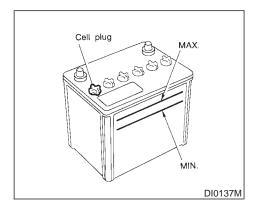
Check the fluid level in each cell. It should be between the MAX. and MIN. lines.
