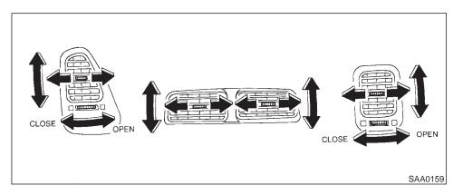
Open or close, and adjust the air flow direction of ventilators.
