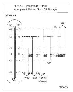
75W-90 for transfer, and 80W-90 for differential are preferable if the ambient temperature is below 104°F (40°C).
