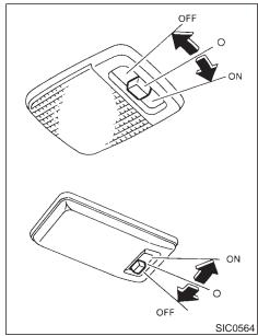
The interior light has a three position switch.
