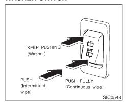
To operate the wiper, push the switch to the side. This wiper operates intermittently. Push the switch to the \subseteq side fully, this operates the wiper continuously.
