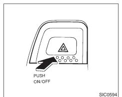
Push the switch on to warn other drivers when you must stop or park under emergency conditions. All turn signal lights will flash.
