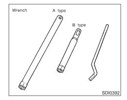
2. Remove spark plugs with a spark plug wrench. (Type A or B)
