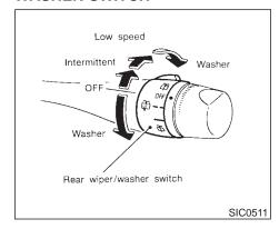
The rear window wiper and washer operates when the ignition switch is in the ACC or ON position.
