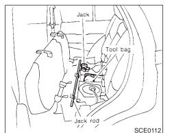
Stowing the damaged tire and tools
