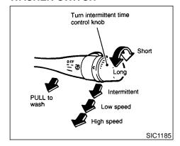
The windshield wiper and washer operates when the ignition key is in the ACC or ON position.
