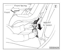
Route the seat belt tongue through the child restraint and insert it into the buckle until you hear and feel the latch engage. Be sure to follow the child restraint manufacturer's instructions for belt routing.
