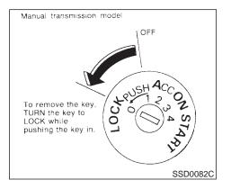
To lock the steering wheel, remove the key. To unlock the steering wheel, insert the key and turn it gently while rotating the steering wheel slightly right and left.
