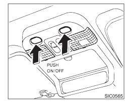
When the interior light or the personal light switch is in the ON position, the interior, personal, and vanity mirror lights will automatically turn off 10 minutes after the ignition switch has been turned to the OFF position. To turn on the light again, insert the key into the ignition switch and move it to the ON position.
