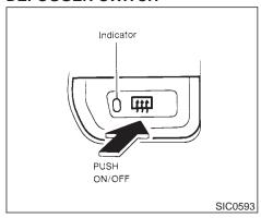
To defog the glass hatch and the outside door mirrors, start the engine and push the switch on. (The indicator light will come on.) Push the switch again to turn the defogger off.
