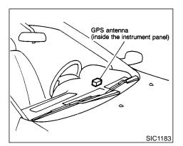
Avoid placing objects over the GPS antenna installed inside the vehicle and do not place portable telephones and hand held wireless units near the Nissan Communicator antennas. Also, keep the front and/or rear windshield free of snow and ice. Since the strength of radio waves from the GPS satellites is relatively small, signal quality may drop, resulting in poor or no signal reception.
