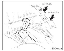
**2H** — (2WD, high range) Only the rear wheels are driven. Use when driving under the same conditions as standard 2WD vehicle.
