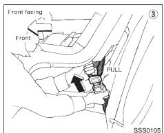
Remove all slack in the lap belt for a very tight fit by pulling forcefully on the lap belt adjustment.
