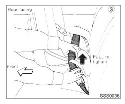
3. Remove all slack in the lap belt for a very tight fit by pulling forcefully on the lap belt adjustment.
