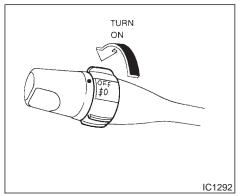
To turn the fog lights on, turn the headlight switch to the  $\underset{\bigcirc}{\text{|c|}}$  position, then turn the switch to the  $\underset{\bigcirc}{\text{|c|}}$  position. To turn them off, turn the switch to the OFF position.
