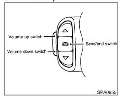
You can receive phone calls and also adjust the volume during the conversation. To receive a phone call, press the send/end switch. The audio system automatically turns off (auto mute) during the call. Press the send/end switch to end the call. The audio system will automatically turn on in about four seconds.
