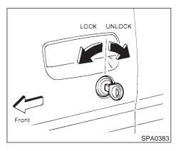
• Turning the front door key one time to the rear of the vehicle will unlock the corresponding door. From that position, returning the key to neutral (where the key can only be removed and inserted.) and turning it to the rear again within 5 seconds will unlock all doors.
