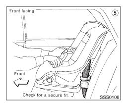
seat belt is allowed to wind back into the retractor, the automatic locking mode (child restraint mode) is canceled; the seat belt only locks during a sudden stop or impact.
