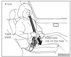
you could be thrown into it and receive neck or other serious injuries. You could also slide under the lap belt and receive serious internal injuries.
