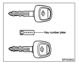
You can only drive your vehicle using the master keys which are registered to the Nissan Vehicle Immobiliser System components in your vehicle. These keys have a transponder chip in the key head.
