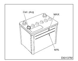
Check the fluid level in each cell. It should be between the MAX. and MIN. lines.
