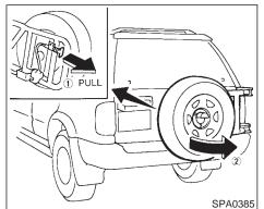
When opening the back door, first open the spare tire carrier in the sequence shown in the illustration above. Then insert the stopper into the hole to secure the carrier in the open position.
