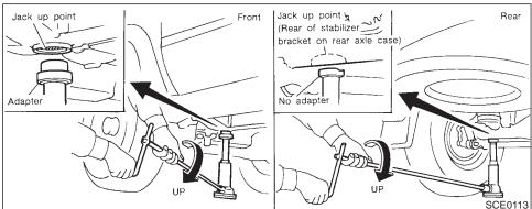
Jacking up the vehicle and removing the damaged tire
