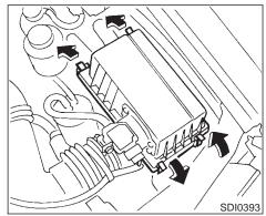
The filter element should not be cleaned and reused as it is given a special treatment. We recommended it be replaced according to the maintenance intervals. See "Periodic maintenance" in the "9. Maintenance" section for maintenance intervals. When replacing the filter, wipe the inside of the air cleaner housing and the cover with a damp cloth.
