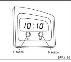
The digital clock displays time when the ignition key is in ACC or ON.
