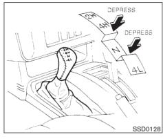
2H - (2WD, high range) Only the rear wheels are driven. Use for driving under the same conditions as standard 2WD vehicle, or state dynamometer I/M testing.
