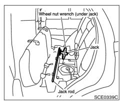
5. Securely store the tire and jacking equipment in the vehicle as illustrated.
