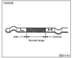
remove the oil filler cap and pour recommended oil through the opening. Do not overfill.
