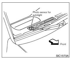
Be sure not to put anything on top of the photo sensor located on the top right-hand side of the instrument panel. The photo sensor controls the autolight; if it is covered, the photo sensor reacts as if it is dark and the headlights will illuminate.
