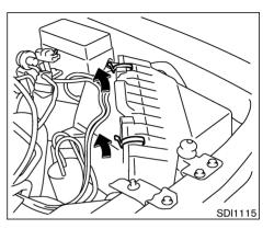
The filter element should not be cleaned and reused as it is given a special treatment. We recommended it be replaced according to the maintenance log shown in a separate "Service and Maintenance Guide". When replacing the filter, wipe the inside of the air cleaner housing and the cover with a damp cloth.
