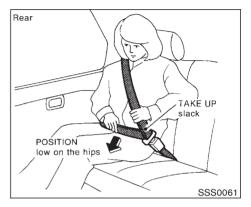
The front seat passenger side seat belt and rear three-point seat belts have a cinching mechanism for child restraint installation. It is referred to as the automatic locking mode.
