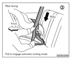
Pull on the shoulder belt until all of the belt is fully extended. At this time, the belt retractor is in the automatic locking mode (child restraint mode). It reverts back to emergency locking mode when the belt is fully retracted.
