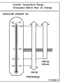
SAE 5W-30 viscosity oil is preferred for all ambient temperatures. SAE 10W-30, 10W-40 viscosity oil may be used if the ambient temperature is above  $0^{\circ}F(-18^{\circ}C)$ .
