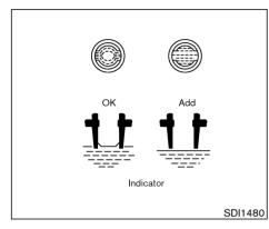
under severe conditions require frequent checks of the battery fluid level.
