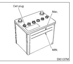
Check the fluid level in each cell. It should be between the MAX. and MIN. lines.
