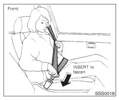
THREE-POINT TYPE SEAT BELT WITH RETRACTOR
