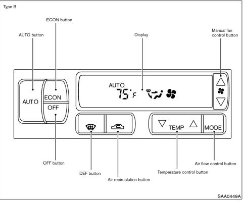
Start the engine and operate the controls to activate the air conditioner.
