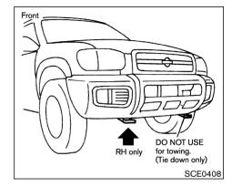
VEHICLE RECOVERY (Freeing a stuck vehicle)
