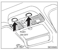
When the interior light or the personal light switch is in the ON position, the interior, personal, and vanity mirror lights will automatically turn off 30 minutes after the ignition switch has been turned to the OFF position. To turn on the light again, insert the key into the ignition switch and move it to the ON position.
