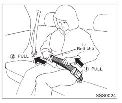
2. To lengthen, hold the tongue at a right angle to the belt and pull on the belt.
