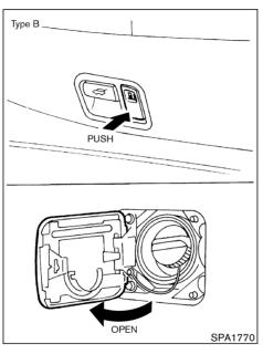
The fuel filler lid release switch is located on the floor below the driver's arm rest.
