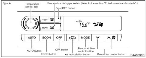
Start the engine and operate the controls to activate the air conditioner.
