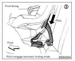
3. Pull on the shoulder belt until all of the belt is fully extended. At this time, the belt retractor is in the automatic locking mode (child restraint mode). It reverts back to emergency locking mode when the buckle is unlatched and the belt is allowed to fully retract.
