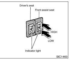
The front seat(s) are warmed by built-in heaters. The switches located on the instrument panel can be operated independently of each other.
