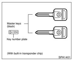
You can only drive your vehicle using the master keys which are registered to the Nissan Vehicle Immobilizer System (NVIS) components in your vehicle. These keys have a transponder chip in the key head.
