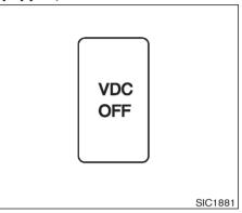
The vehicle should be driven with the Vehicle Dynamic Control System (VDC) on for most driving conditions.
