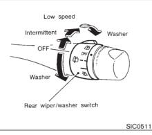
The rear window wiper and washer operates when the ignition switch is in the ON position.
