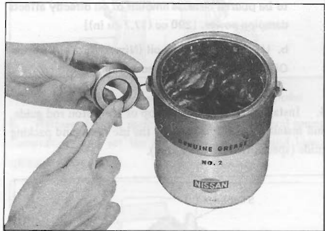
Fig. FA-33 Greasing strut mounting bearing
