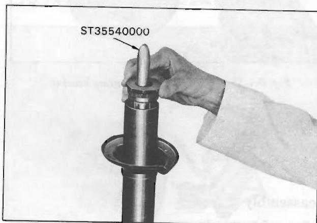
Fig. FA-35 Installing gland packing
