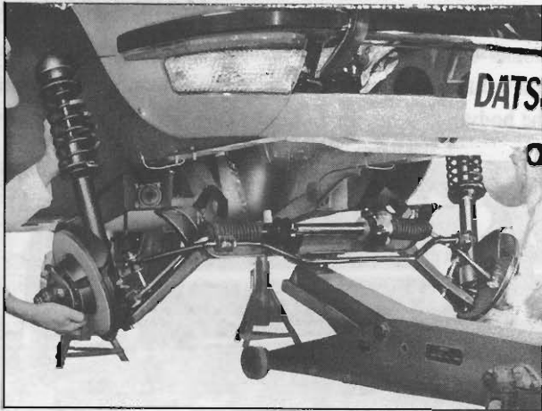
Fig. FA-11 Removing front axle and suspension assembly
