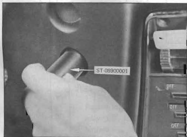
Fig. BE-31 Removing switch
