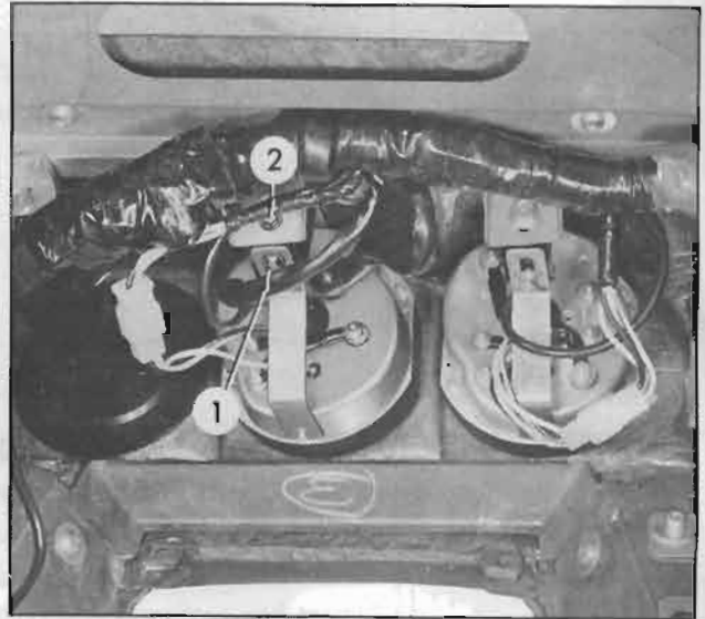
Fig. BE-22 Removing ammeter and fuel gauge
