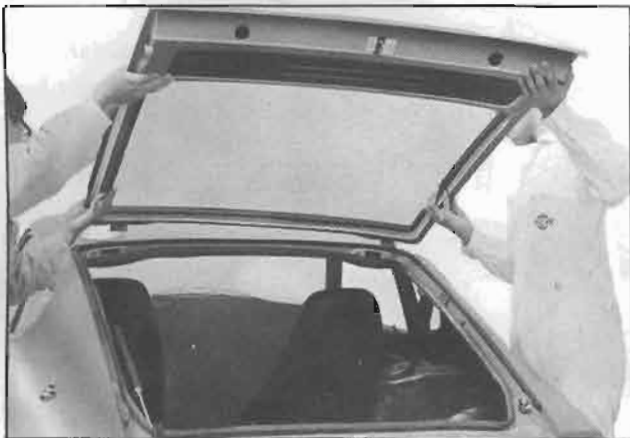
Fig. BF-41 Removing tail gate
