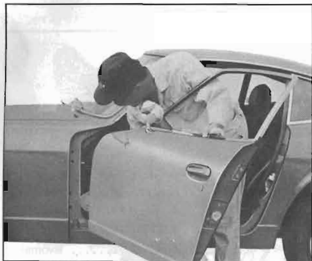
Fig. BF-22 Removing the door
