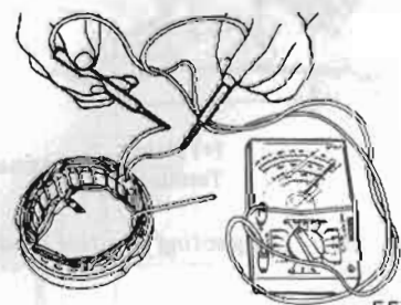
EE043 Fig. EE-44 Testing stator for conduction
