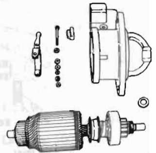
Fig. EE-13 Removing armature assembly and shift lever
