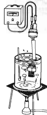
Fig. ET-60 Checking water temperature switch operation
