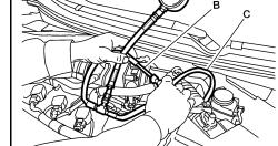
If result is unsatisfactory, check fuel hoses and fuel tubes for clogging.
