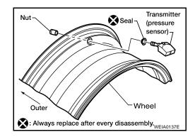
2. Mount transmitter on rim and tighten nut to specification.
