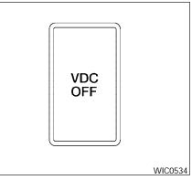
The vehicle should be driven with the Vehicle Dynamic Control (VDC) system on for most driving conditions.
