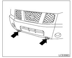
VEHICLE RECOVERY (freeing a stuck vehicle)
