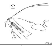
The sunload sensor ①, located on the top center of the instrument panel, helps the system maintain a constant temperature. Do not put anything on or around this sensor. To operate the rear air conditioner, the engine must be running.
