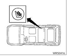
LATCH system anchor point locations 2nd row bench seat (if so equipped)
