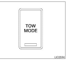
Tow mode should be used when pulling a heavy trailer or hauling a heavy load. Using tow mode at other times may cause unnecessary transmission shifting and reduced fuel economy.
