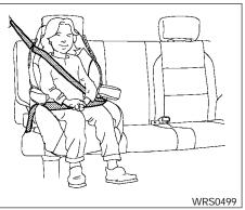
(Outboard position) BOOSTER SEAT INSTALLATION ON 3RD ROW BENCH SEAT POSITIONS
