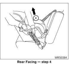
(4) Allow the seat belt to retract. Pull up on the shoulder belt to remove any slack in the belt.
