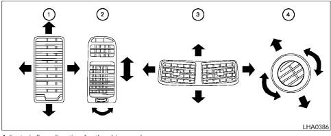
Adjust air flow direction for the driver and passenger side (1), center (2), and rear passenger (3) and (4) ventilators by moving the ventilator slide and/or ventilator assemblies.
