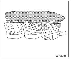
Supplemental side-impact air bag (if so equipped) and curtain side-impact and rollover air bags system
