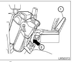
Then ② lift up on the lower corner of the seat base and tip the 2nd row captain's chair forward. To exit the 3rd row bench seat lift up on the same latch and fold the seatback forward onto the seat base. Then lift up on the seat base and tip it forward.
