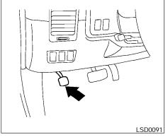
To engage: Firmly depress the parking brake.
