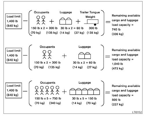
Steps for determining correct load limit
