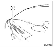
Be sure you do not put anything on top of the autolight sensor ① located in the top side of the instrument panel. The autolight sensor controls the autolight; if it is covered, the autolight sensor reacts as if it is dark out and the headlights will illuminate. If this occurs while parked with the engine off and the key in the ON position, your vehicle's battery could become discharged.
