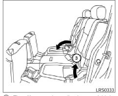
(3) Then lift up on the recline lever to fold the seatback flat forward.
