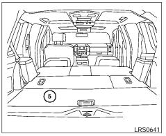
(5) The carpet panel flaps provide a level cargo floor when the 3rd row seats are also folded flat. Reverse this process to return the 2nd row captain's chairs to a seating position. Make sure to properly raise the seatback to an upright position and push the seat cushion down into place.
