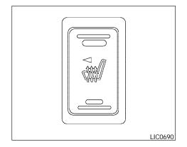
The front seats are warmed by built-in heaters (if so equipped).
