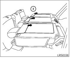
③ There is a carpet panel flap on the back of each seat that can be folded toward the back of the vehicle
