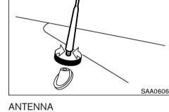
The antenna is located at the rear of the vehicle. To remove the antenna, turn it counterclockwise, To reinstall it, screw it securely into the base.
