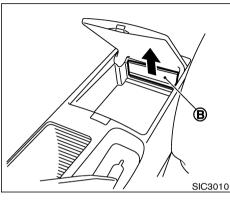
If objects (coins, etc.) fall into the rear section of the center console box, remove the rear wall (B) of the box as shown, and pick up the objects.
