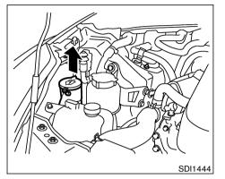
Open the cap and add fluid when the low washer fluid warning light comes on.
