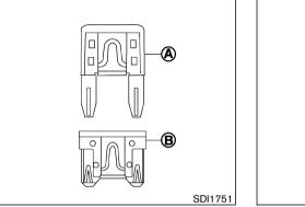
Some vehicles are equipped with engine compartment and passenger compartment fuse boxes that use only type (A) fuses. Other vehicles are equipped with type (A) fuses in the engine compartment fuse box and type (B) fuses in the passenger compartment fuse box.
