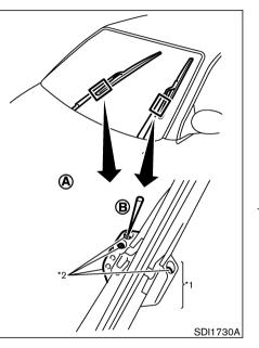
If necessary, clean the windshield washer nozzle (A) with a needle or small pin (B).
