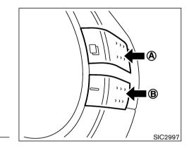
Switches for the trip computer are located on the side of the combination meter panel. To operate the trip computer, push the side of the switches as shown above.
