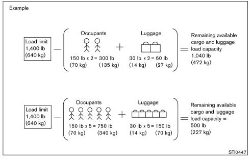
Steps for determining correct load limit
