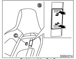
Roadster models – Type B seatback tilt switch. While the switch is held down, the seatback will move backward to the original position that was last selected using the reclining switch (located on the seat cushion). Release the switch to stop the movement.
