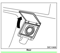
rear power outlets. Do not use double adapters or more than one accessory with a single power outlet.
