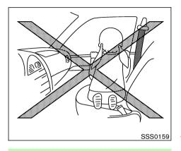
• The seat belts, the supplemental side air bags and curtain side-impact air bags are most effective when you are sitting well back and upright in the seat. The side air bag and curtain side-impact air bag inflate with great force. Do not allow anyone to place their hand, leg or face near the side air bag on the side of the seatback of the front seat or near the side roof rails. Do not allow anyone sitting in the front seat to extend their hand
