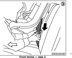
3. Route the seat belt tongue through the child restraint and insert it into the buckle until you hear and feel the latch engage. Be sure to follow the child restraint manufacturer's instructions for belt routing.
