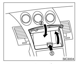
INSTRUMENT POCKET (except for navigation system equipped models) To open the lid, push the knob up (1).
