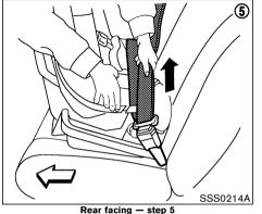
5. Allow the belt to retract. Pull up the belt to remove any slack in the belt.
