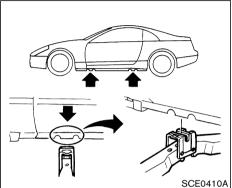
Jack-up point Jacking up the vehicle and removing the damaged tire
