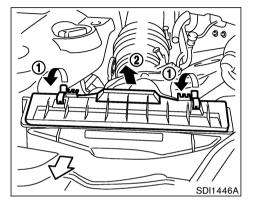
To remove the filter from the air cleaner, pull off the lock pins (1) and pull the unit upward (2).
