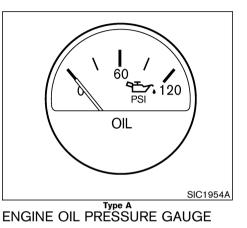
The gauge indicates the engine lubrication system oil pressure while the engine is running. When the engine speed is high, the engine oil pressure is also high. When it is low, the gauge indicates the low oil pressure.
