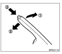
**To apply:** pull the parking brake lever up (1).
