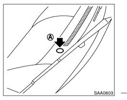
Sensor (A) on the instrument panel helps maintain a constant temperature; do not put anything on or around this sensor.
