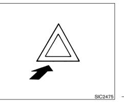
Push the switch (located on the front part of the center console) on to warn other drivers when you must stop or park under emergency conditions. All turn signal lights will flash.
