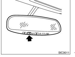
Using both hands, simultaneously press and hold both the HomeLink<sup>®</sup> button you want to program and the hand-held transmitter button.
