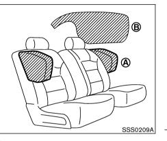
Supplemental side air bag and curtain side-impact air bag systems (if so equipped)
