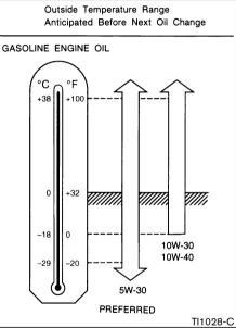
SAE 5W-30 viscosity oil is preferred for all ambient temperatures. SAE 10W-30 or 10W-40 viscosity oil may be used if the ambient temperature is above  $0^{\circ}F(-18^{\circ}C)$ .
