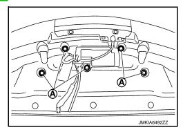
3. Remove harness grommet (A), and then disconnect harness connector (B).
