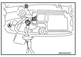
4. Remove solar cell module from rear spoiler.
