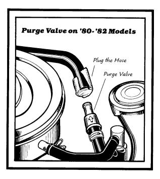
and pull the hose off the fitting. Use tape, a cork, or whatever to plug the open end of the hose.
