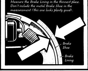
If the shoes, drums, and wheel cylinder are OK, go on to Step 3 and install the drums, then do Step 4 to tighten the axle nuts.
