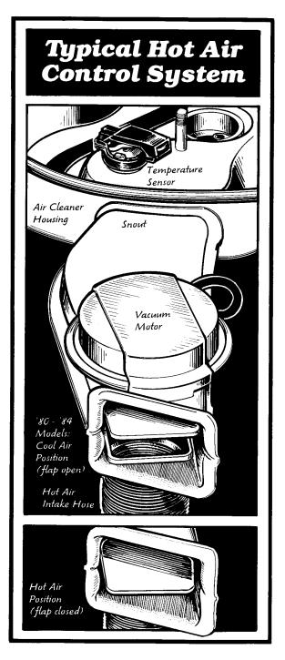
Drawing warm air into the carb in cold weather also shortens engine warm-up time and helps prevent carburetor icing.
