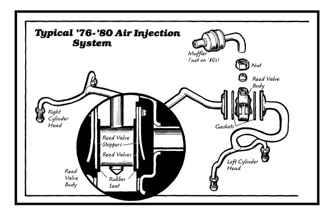
the hose sucking on your finger, not pressure trying to blow your finger off the hose. If you feel pressure, the *air injection valve* needs replacing (Step 3).
