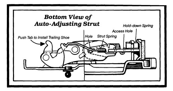
**Auto-adjust models:** After the drums and wheels are on, lower the car to the ground, then pump on the brake pedal several times. This adjusts the rear brake shoes.
