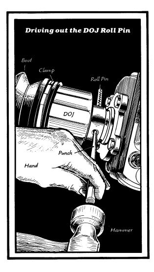
and remove the spare tire if you haven't already. Rotate the right wheel until you see the roll pin in the small part of the DOJ. Use a 5/32" or 3/16" (5mm or 6mm) punch and hammer to tap the roll pin out far enough so the DOJ can slide toward the front wheel.
