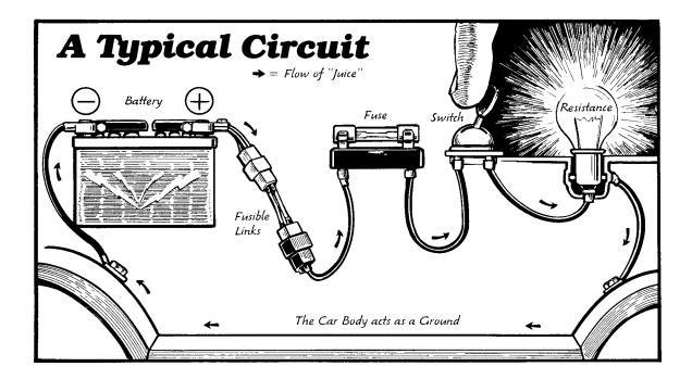
links on '78 and newer models are installed in each circuit, with one exception-the cranking circuit. Fuses and fusible links are made of lighter, more fragile material than the wires and components in the circle. They're designed to melt and break if more juice is flowing through the circuit than the wires or components can handle.
