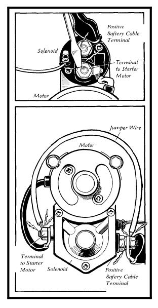
Checking the Starter Solenoid and Motor (second test)
