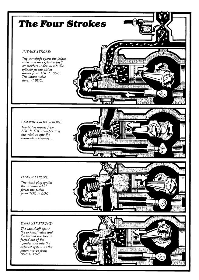
1. **Intake stroke:** The intake valve opens as the piston moves from TDC to BDC and the fuel-air vaporous mixture is sucked into the increasing space inside the cylinder (like sucking fluid into a syringe). When the piston reaches BDC, the intake valve closes.
