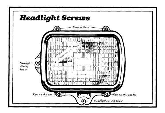
Step 1. Replace Headlight (and parking and turn signal bulbs on some '80 and newer OHV models).
