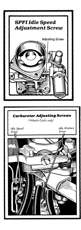
Idle Speed Adjustment Screw: Here's where to find it:
