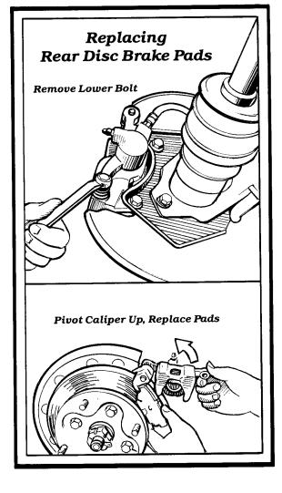
and over the pads. Install the lower mounting bolt and tighten it to 16-23 ft. lbs. Skip down to Step 6 to finish the job.
