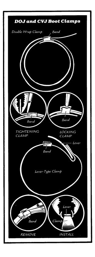
large hose clamps. You can use hose clamps in place of the boot clamps everywhere except for the large clamp on the left front DOJ, where there isn't enough clearance for the clamp screw to rotate between the DOJ and the steering gear. If you use hose clamps, use the ones with the smallest clamp screw you can find.
