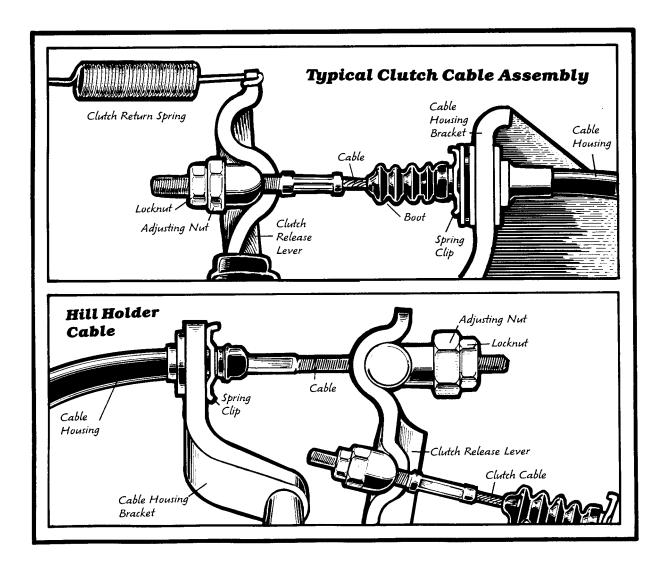
nut *clockwise* (as viewed from the front of the car) to decrease the free play. Turn the 14mm nut a turn or two, then check the pedal free play again. Keep turning the nut and checking until you have the proper free play.
