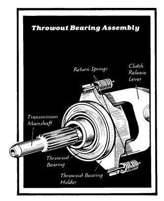
Check the old bearing to see which side was out, then use a punch or screwdriver and hammer to tap the new bearing onto the holder the same way. Only tap on the thick inner race of the bearing, not on the rounded part. Tap it on all the way.
