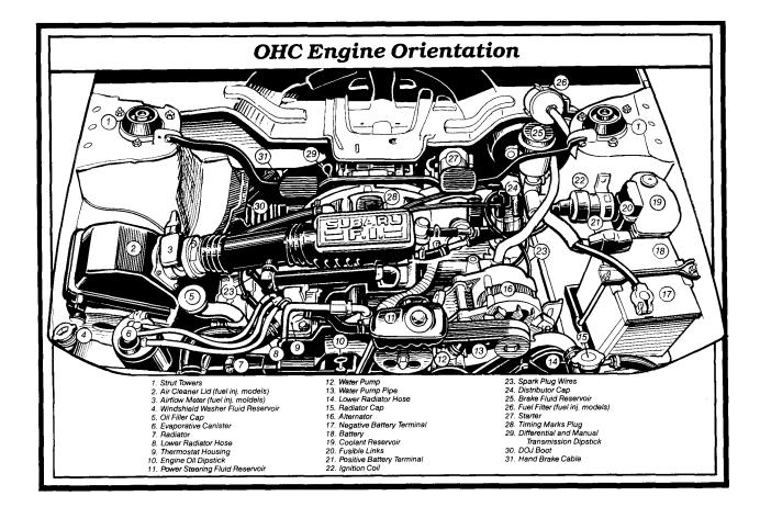
The water pump is bolted to the left front of the engine. A pulley on the front of the water pump is driven by a drive belt from the nearby crankshaft pulley.
