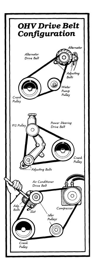
Adjust drive belt: Slightly loosen the 12mm tension adjusting bolt and the pivot bolt(s) if you haven't already.
