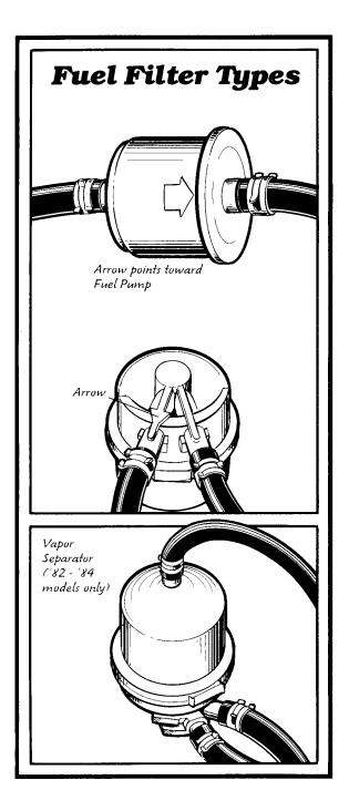
Step 1. Locate and Check Fuel Filter.
