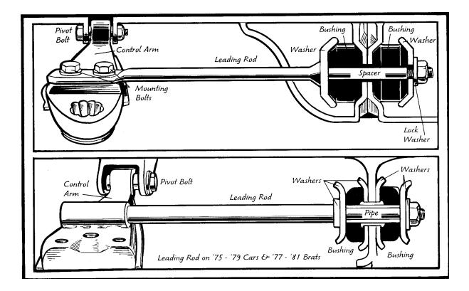
the rod around until you're sure it's centered. Torque the nut to 60 ft. lbs.
