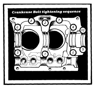
the torque pattern and torque the 12mm and 14mm bolts and nuts to 20 ft. lbs. Also torque the 12mm pickup tube bolt on the bottom to 20 ft. lbs. Finally, follow the pattern and torque only the 14mm nuts or bolts to 35 ft. lbs. Do the final pattern at least twice.
