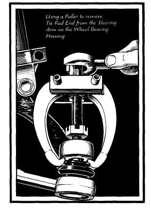
end anyway, unscrew the castle nut, turn it over so the notched part is facing down and screw it onto the ball joint until the top of the nut is even with the top of the bolt. Put a block of wood on the top of the nut, then hit the block SQUARELY with the hammer and the ball joint will pop out. Remove the castle nut. If the stud turns with the nut, lightly tap the ball joint backup into the arm and hold it there while you unscrew the castle nut.
