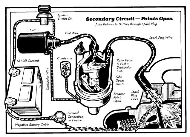
Electricity, like water, will follow the path of least resistance, so if one path is closed, it will follow another. A small cylinder, called the condenser, located on the outside of the distributor, is part of the path while the points are open (not touching). The condenser stops the 12 volt current and keeps it from jumping the point gap to get to the distributor body. This stopping of the current also prevents the points from burning and pitting too rapidly.
