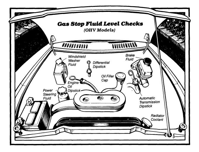
Pull out the dipstick again. The oil on the stick should stop somewhere between the two little holes in the dipstick. If the oil level is on or below the bottom hole, add one U.S. quart (0.95 liters) of oil. Use the same kind of oil you already have in your engine. After adding the quart, check the level again.
