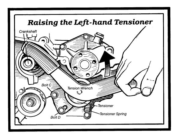
without moving the handle while you (or Friend) snugs down bolt D (the lower bolt) and then bolt C (the upper bolt). After both bolts are snug, put the socket on the torque wrench and torque bolt D, then bolt C to 14 ft. lbs. Check both bolts again. The left belt is adjusted. Wasn't too hard, eh?
