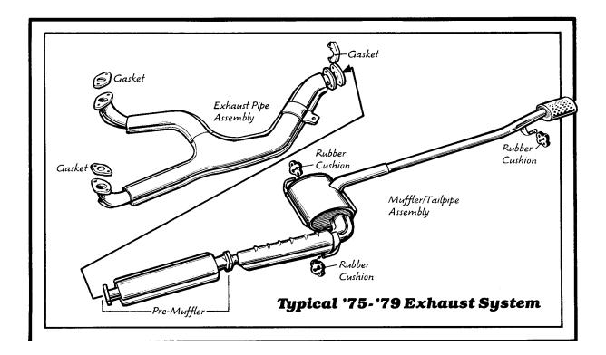
Step 2. Replace Exhaust Pipe Assembly and/or the Gaskets between the Cylinder Head and Exhaust Pipe (non-Turbo models).
