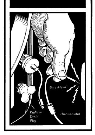
Still no fan? Remove the two phillips head screws that attach a short piece of wire to the top right side of the radiator and to the body in front of the radi ator. Clean the ends of the wire and the area around the screw holes with emery paper until the metal is clean and bright. Put the wire and screws back in place and tighten them. Start the engine again to see if the fan goes on when the temperature gauge crosses the halfway mark.
