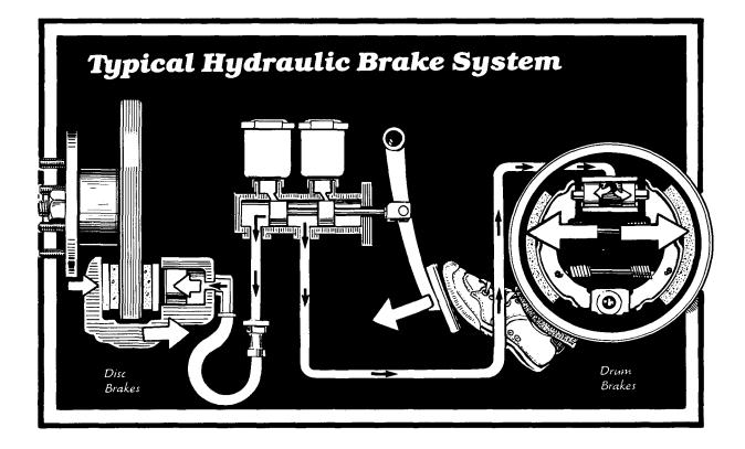
These wheel (or "slave") cylinders are bolted to brackets near the end of each axle. A short rubber brake hose takes the place of the metal lines near each wheel, allowing the wheels to move up and down and the front wheels to turn right and left.
