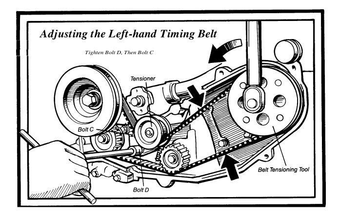
We'll adjust the left-hand belt first. Loosen bolts C and D about 1/2 turn *counterclockwise* (as viewed from the front of the car). Look at the illustration "Adjusting Left-Hand Timing Belt." Watch the tensioner while you squeeze the belt together where the arrows are pointing at the belt. (Your hands are clean, right?) The tensioner should be free enough to move a little. If not, loosen bolts C and D a little more.
