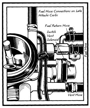
slide it away from the carb. Grab the hose close to the fitting on the carb and twist and pull it off. Cut the top off a 12-ounce beer or pop can and stick the hose into the can.
