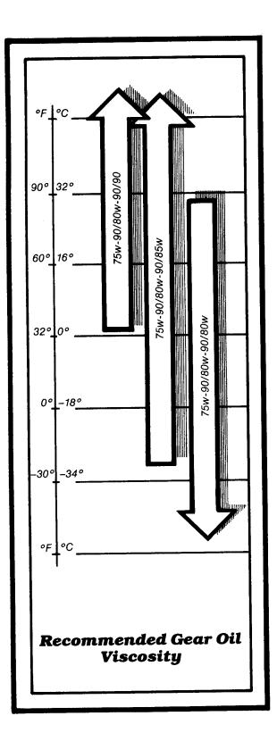
oil is not recommended for sustained high speed driving or for use in Turbo models, so change to one of the oils in the chart as soon as the weather warms up to a balmy  $0^{\circ}$ F (-18°C).
