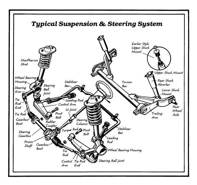
ing up under the front seats every time you hit a curb or ditch, one end of a strong steel rod called a leading rod is attached to the knuckle end of the control arm. The other end of the leading rod is attached securely to the car frame behind the front wheel.
