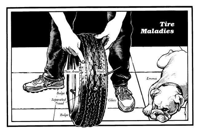
A loss of about 6 psi of pressure between gas stop checks means you have a slow leak that may turn into a fast one rather suddenly. It could be in the valve stem, the valve, the tire, or where the tire seals along the rim of the wheel. Get it fixed. A high speed blowout can kill you dead.
