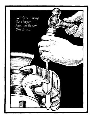
Use needlenose pliers to remove the four tiny hairpin clips located near the outer ends of the stopper plugs. Place a screwdriver against the inner edge of the top stopper plug and tap lightly with a hammer. When the plug is out as fir as you can get it with the screwdriver, try pulling it out with your fingers. Stuck? Put a rag on the plug to protect it, then grab it with pliers and pull it out. Remove the lower stopper plug the same way.
