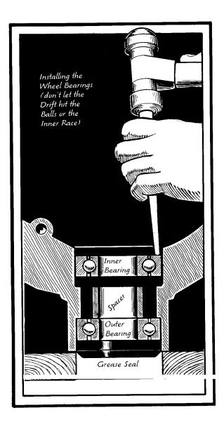
feel it best where the inside of the housing is grooved. Put your "drift" in one of the grooves with the end against the race. Tap the drift lightly with a hammer (see illustration). Move the spacer around so you can tap all the way around the bearing race. Don't let the drift hit the ball bearings or inner race. Don't try to take it out in one punch, Rocky, just keep tapping round and round and soon the bearing will drop out of the housing.
