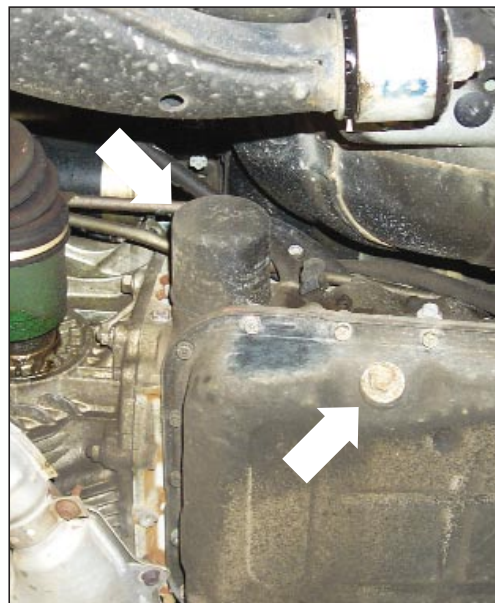
Transmission drain and filter
