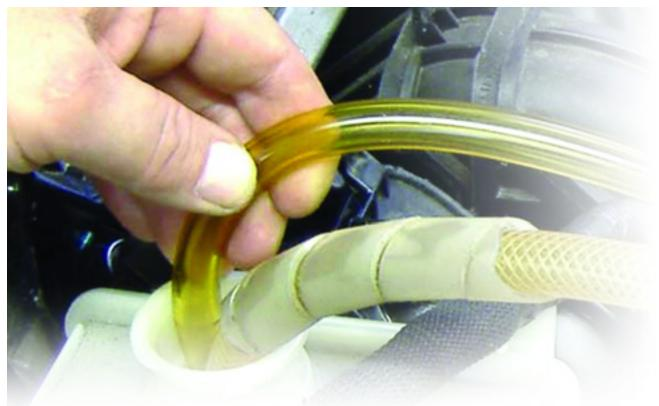
With a flushing machine, one hose extracts the old fluid from the bottom of the reservoir while the other supplies the fresh load.
