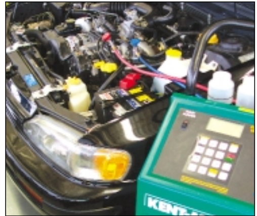
Recovering Refrigerant and Oil
