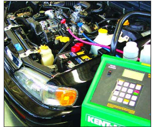
Recovering Refrigerant and Oil
