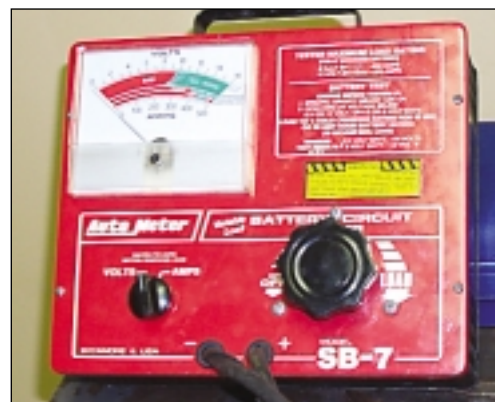
Battery Load Tester
