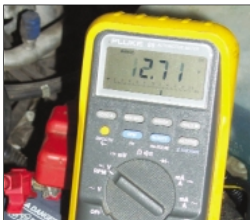
Battery Open Circuit Voltage
