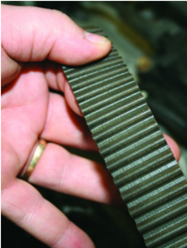
Inspect the timing belt closely for any cracks, wear or erosion of the teeth. Never reinstall a questionable timing belt.
