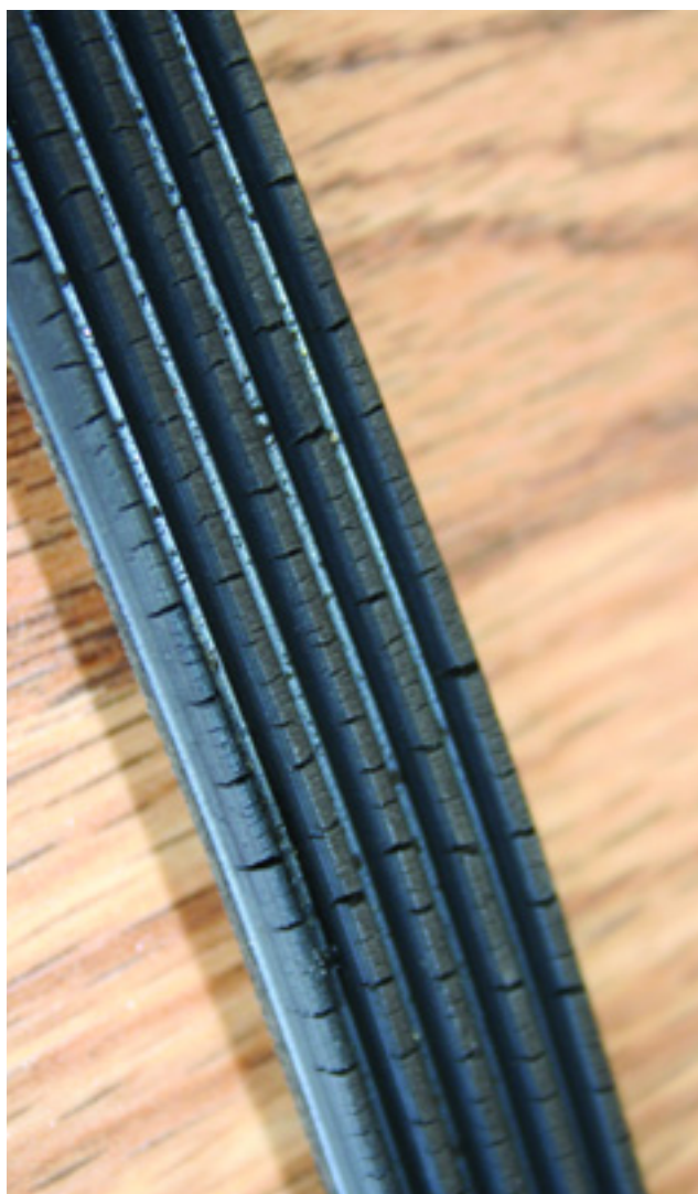
Inspection of accessory drive belts is required every 30,000 miles.
