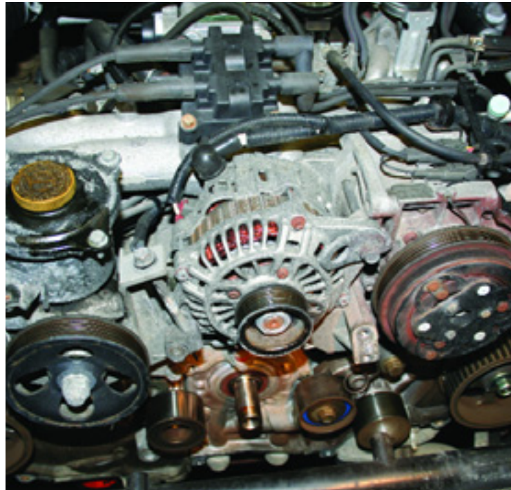
Thorough inspection of all belts, pulleys, tensioners and idlers at the same time is critical to optimum performance of the entire system.
