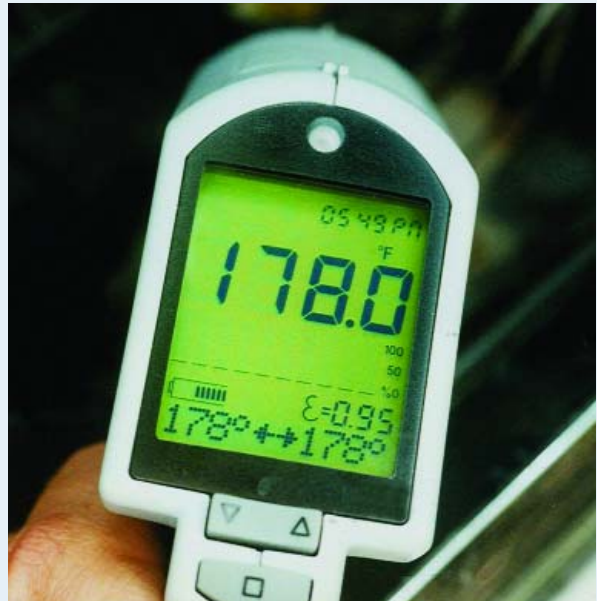
By showing you the pattern of heat dissipation in the radiator, a non-contact infra-red pyrometer can help you find blockage, but it's not a sure thing.
