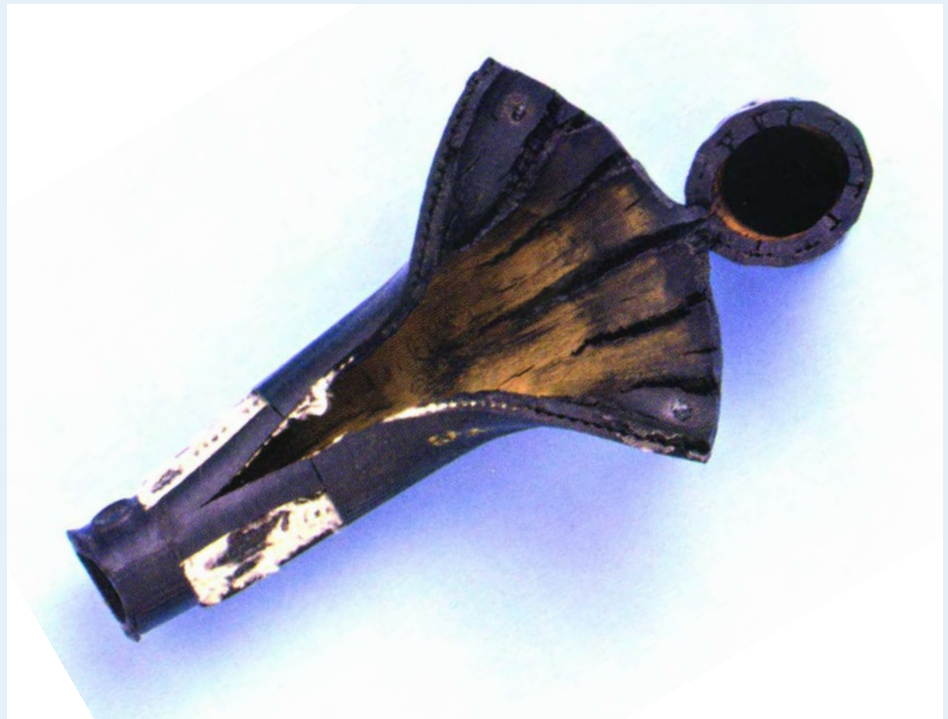
This is a textbook example of how hoses deteriorate. It's actually an electro-chemical reaction that causes the damage. This one was on the verge of blowing and perhaps causing an engine-killing overheating incident.
