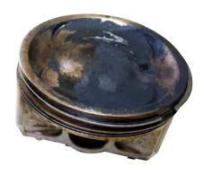
> These pistons were damaged by an overheated engine. Extensive repairs were required to put the vehicle back on the road.
