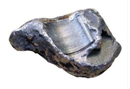
> These used to be pistons. When the gaskets blew, so did the entire engine.
