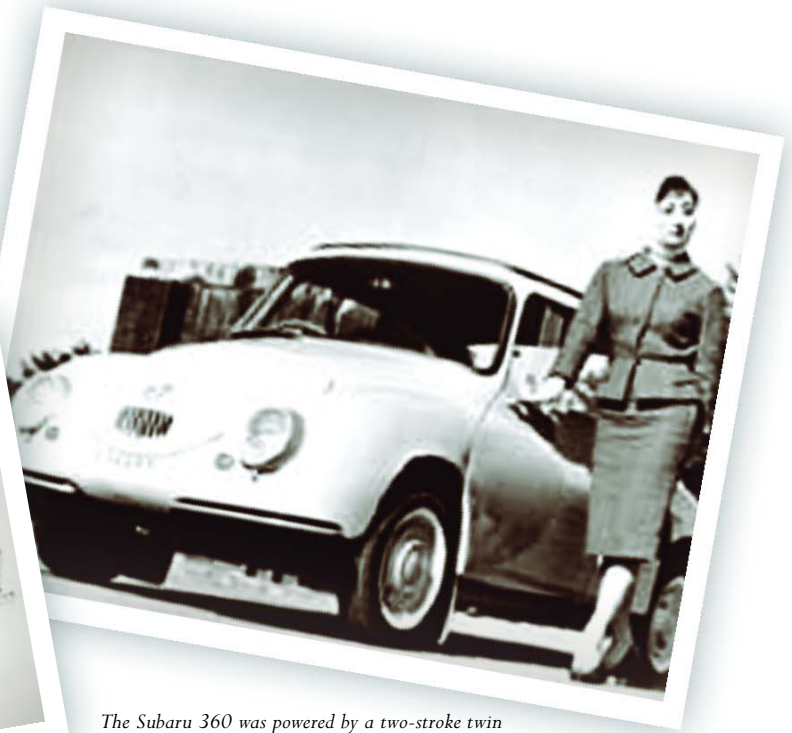
The Subaru 360 was powered by a two-stroke twin and got 66 mpg. It was imported into the U.S. starting in 1968.
