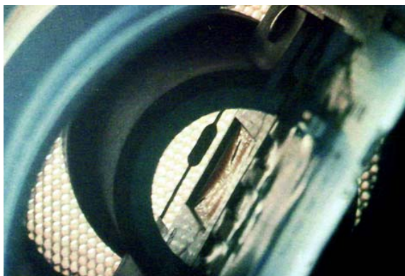
Left: A look down the throat of an early Subaru MAF, circa 1985 or so.
