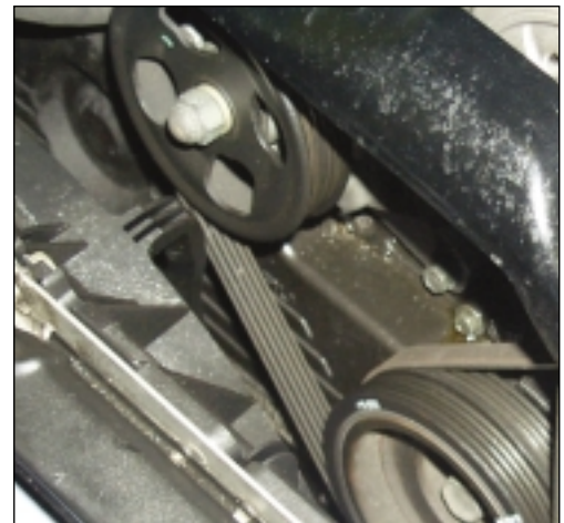
Drive Belt Inspection
