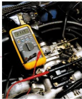
Figure 2 Measuring Secondary Resistance Between Terminals 3 and 4
