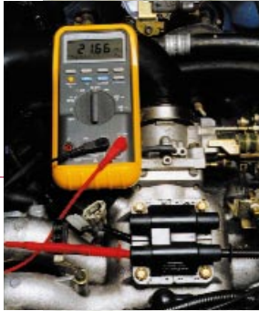
Figure 1 Measuring Secondary Resistance Between Terminals 1 and 2
