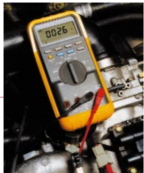
Figure 4 Measuring Primary Resistance Between Terminals 2 and 3
