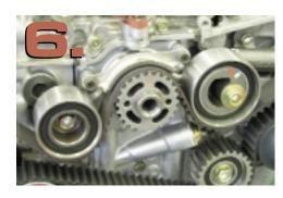
cambelt tensioner, compressing the oil chamber. The tensioner begins to refill the oil chamber after the engine is started and in some cases the tension of the belt was not increased in a timely manner. This would cause the torque of the engine to slip the crankshaft sprocket ahead of the timing belt, creating a crankshaft to camshaft timing problem.
