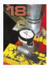
The tensioner rod must be compressed using a hydraulic press. The pressure exerted on the rod must not exceed 66 pounds. Exceeding this pressure may bend the tensioner rod. This will keep the rod from extending fully when it is reinstalled on the engine. If the rod cannot extend fully, excessive slack may develop in the timing belt, causing it to jump teeth. Jumped teeth can mean bent valves or damaged pistons, something you'll certainly want to avoid.
