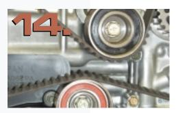
The 2.5 engine's timing belt must negotiate a combination of three idler pulleys, the water pump pulley and the tensioner pulley during each rotation. Pay particular attention to the position and appearance of the different idler pulleys, especially if you happen to
