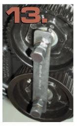
The idler pulley with the least amount of belt tension on it is the lower right idler pulley, which makes it the best candidate for removal when removing the timing belt. This is an all-aluminum engine, so it pays to be careful when removing and installing fasteners. Since the lower pulley isn't under a lot of stress, its mounting bolt can be removed and installed without risk of cross-threading or other damage.
