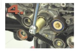
crankshaft, and provides a convenient way to turn the engine over with a breaker bar. Use the tool to turn the crankshaft until all of the timing marks are aligned. This step is especially important because we don't want to try to retime the engine after the timing belt has been removed.
