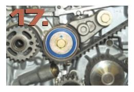
ball and silicone oil. Remove the mounting bolt, then remove the tensioner assembly.
