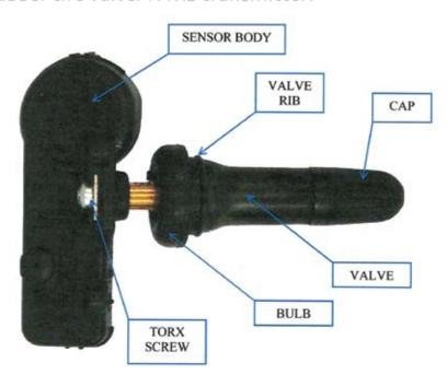
The new "snap-in" valve is made from black rubber and fitted with a black cap. This new valve looks like the older-style valve used on vehicles without TPMS.
