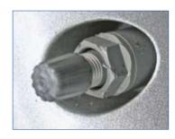
✓ This is the new black rubber tire valve/TPMS transmitter used beginning with 2008 models.
