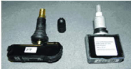
The new rubber-stemmed style of TPMS sensor (left), will replace the old gray style (right) on some 2008 models.
