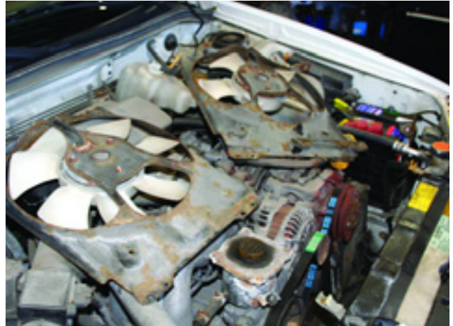
Removing the cooling fans gives you a little more room to swing tools.
