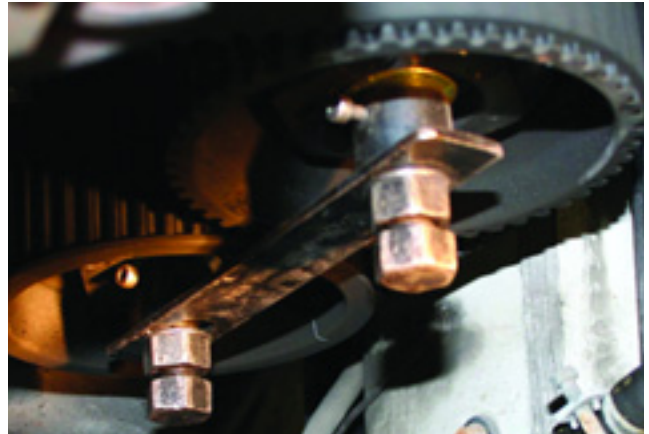
This photo shows the special Cam Sprocket Holder tool in place to prohibit movement of the camshafts.
