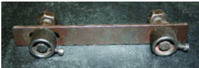
This photo shows the special Cam Sprocket Holder tool in place to prohibit movement of the camshafts.
