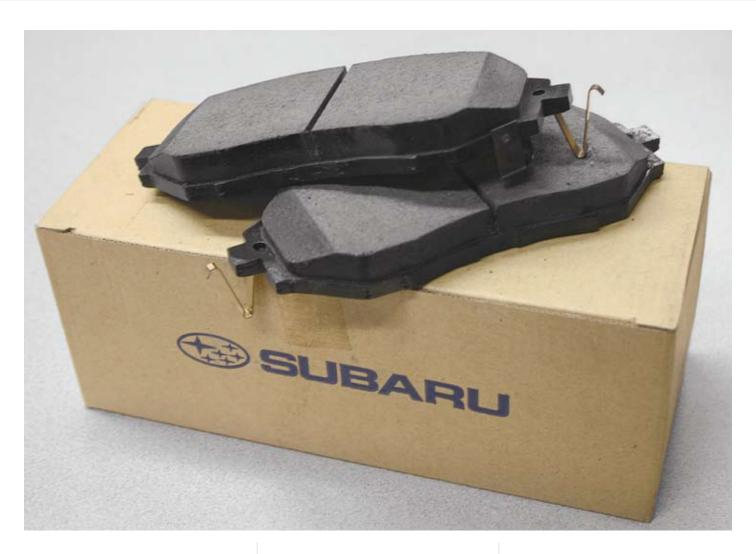
jeopardized. The brake system is then serviced to bring the level of performance – and therefore safety – back up to acceptable standards. Most often, servicing the brake system requires replacing the pads or shoes; usually the rotors or drums must be resurfaced and may often be replaced; and sometimes the calipers require service or replacement.
