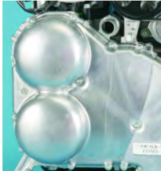
The timing chain cover bulges out to encase the Dual Active Valve Timing System exhaust sprocket.
