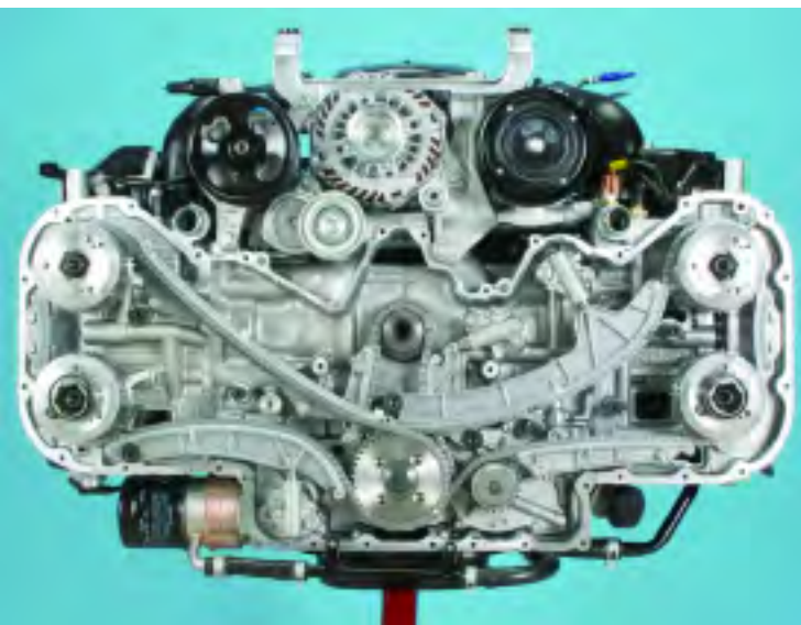
Above: The crankshaft gear drives the idler gear, which then drives the right and left banks.
