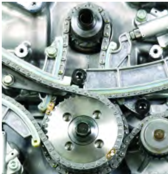
Above: The crankshaft gear drives the idler gear, which then drives the right and left banks.
