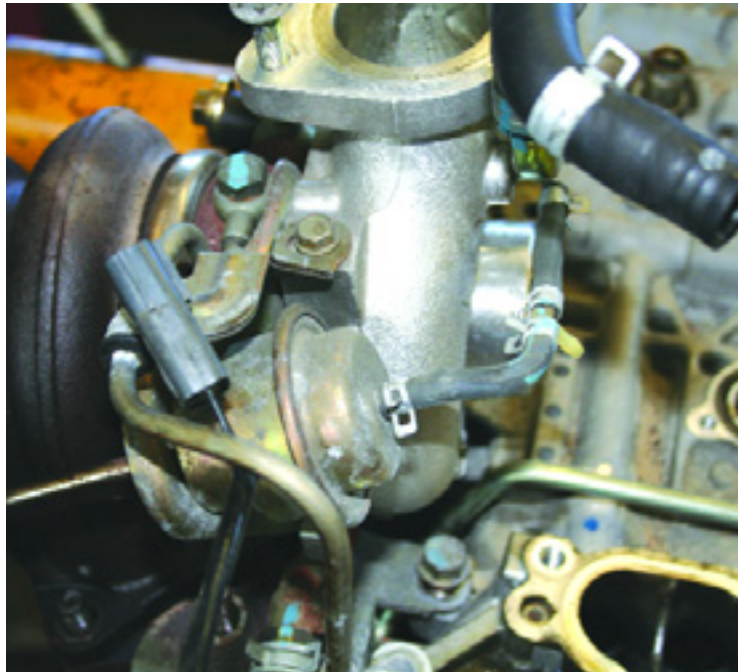
The wastegate controller solenoid is mounted on the side of the turbocharger.
