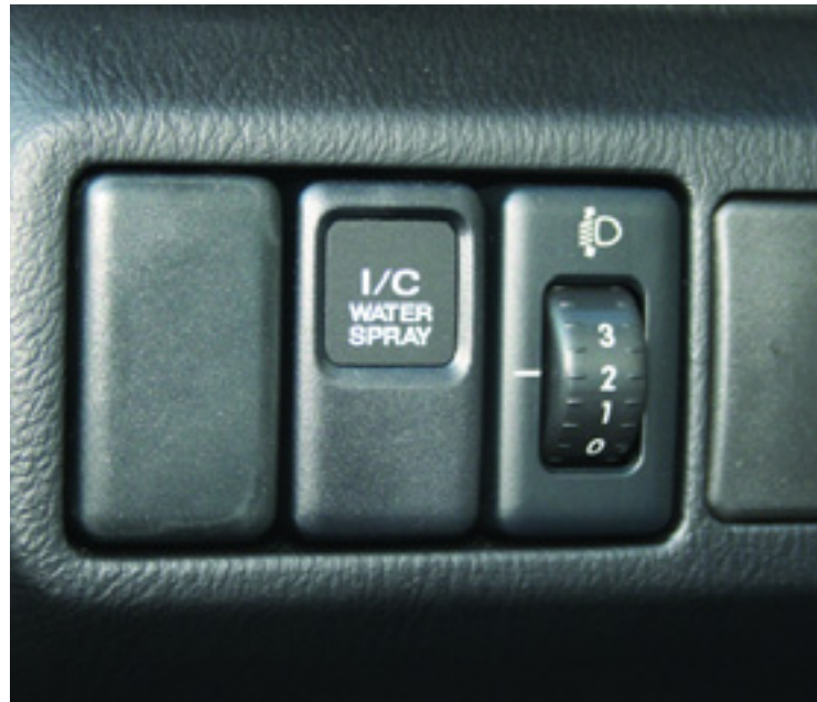
The intercooler water spray system activation button, found on 2004 and later STi models, is located on the left side of the steering wheel.
