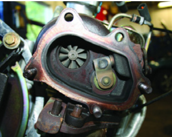
The wastegate valve is located in the turbo exhaust side housing.
