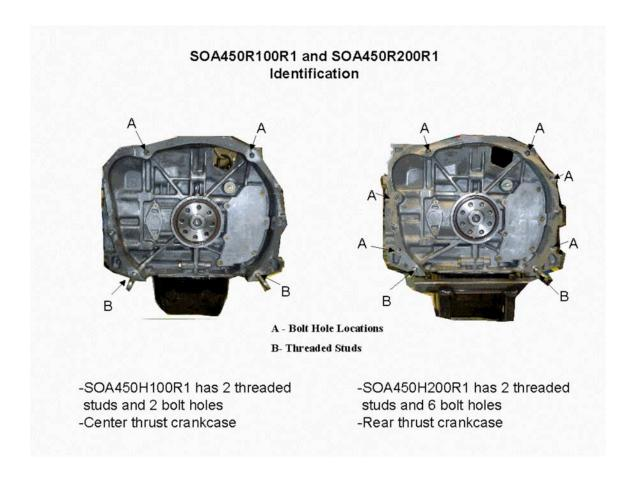
*Note:* You may receive one of two configurations at the outset of the program under part number SOA450H100R1 (a four-hole bolt pattern or an eight-hole bolt pattern). These units are the equivalent in terms of form, fit, and function, and there should be no installation issues.
