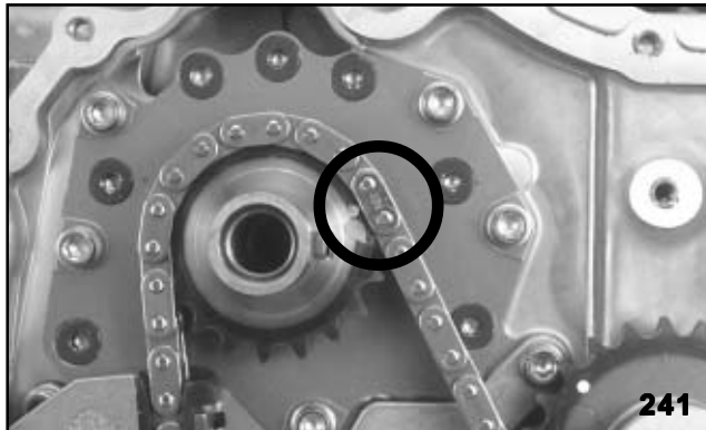
Crankshaft Timing Mark Location
