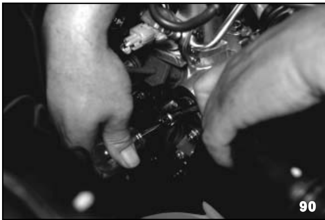
Adjusting Valve Clearance
