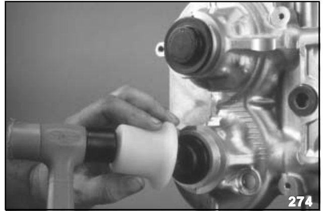
Exhaust Camshaft Oil Seal Installation
