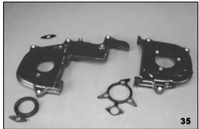
Inner Cam Belt Cover Removal
