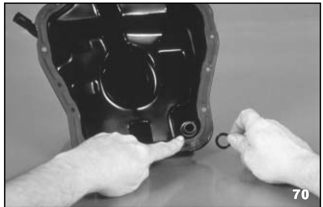
Oil Pan Drain Tube Seal
