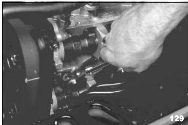
Checking Valve Clearance on the Car
