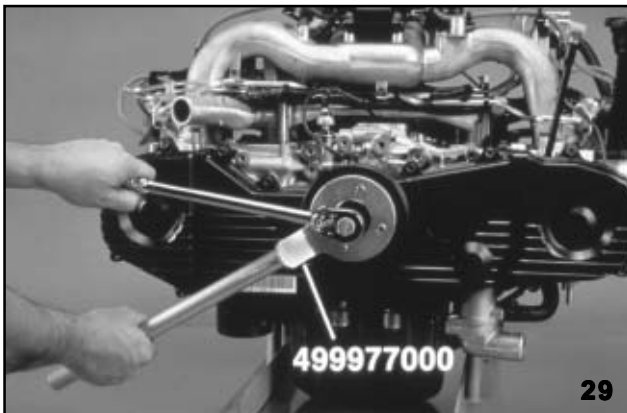
Remove Crank Pulley
