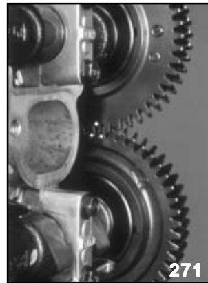
Install Intake Camshaft
