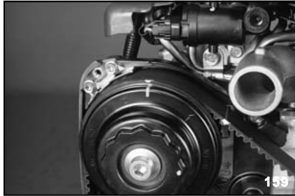
Intake Camshaft Sprocket Timing Marks (Right Bank)
