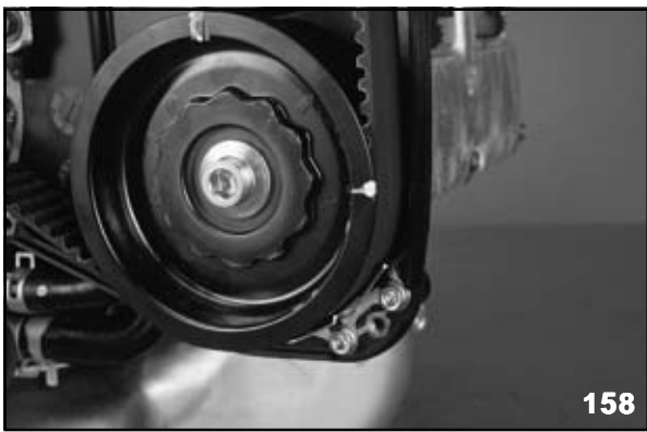
Exhaust Camshaft Sprocket Timing Marks (Left Bank)
