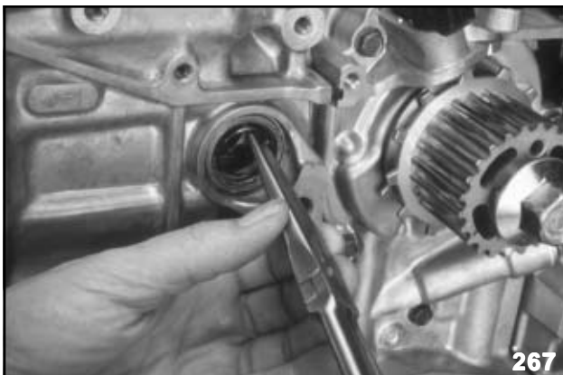
Piston Pin Circlip Removal
