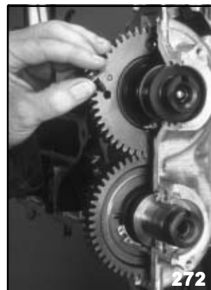
Install Intake Camshaft
