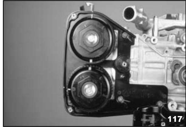
Camshaft Sprocket Timing Marks (Right Bank)
