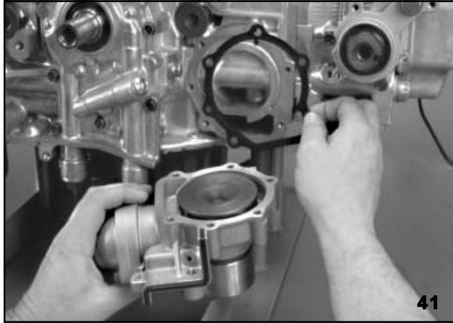
Remove Water Pump
