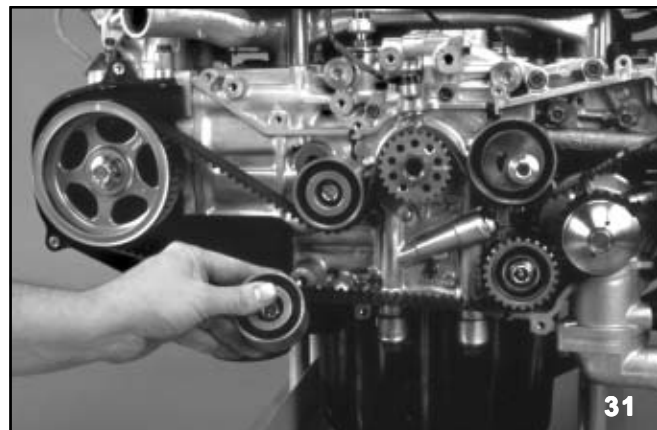
Remove Idler Pulleys
