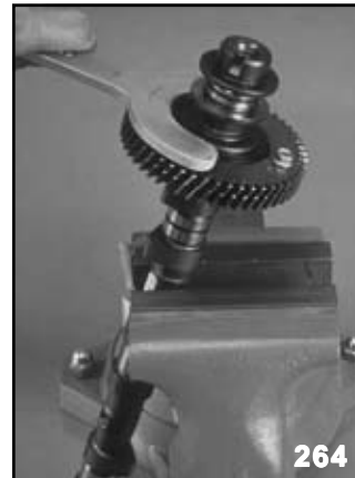
Camshaft Sub-Gear Servicing
