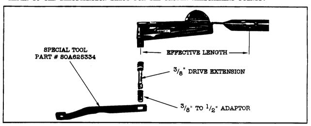
\*SNAP-ON "TORQUEMETER" #TEC12FUA OR EQUIVALENT.
