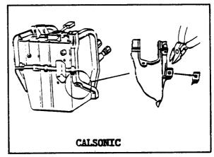
When installing the evaporator assembly, be sure no remaining evaporator case material interferes with the blower case and no air leaks exist.
