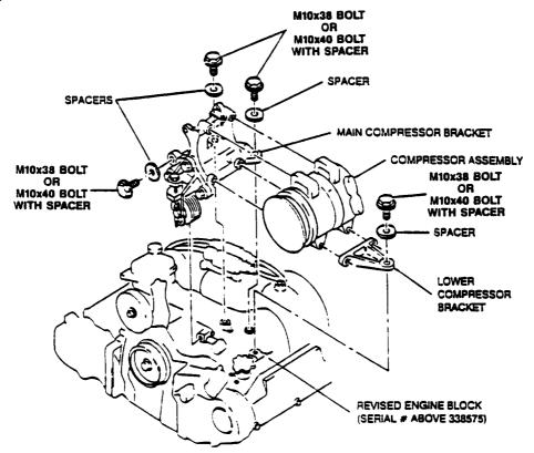
CAUTION: Damage to short block may result if spacer kit or shorter bolts are not used.
