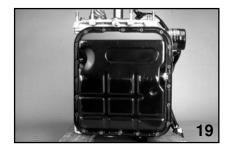
The next step in the disassembly process is to remove the Oil Pan. Position the transmission on the worktable with the Oil Pan facing upward and held in position with wooden blocks.
