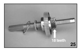
A Sun Gear made on to the end of the Rear Drive Shaft receives the power and transfers the power to the shaft.
