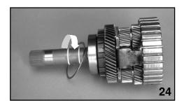
The Pinion Gear is secured to the carrier and delivers power to it. The carrier will now rotate, driving the Reduction Drive Gear. This supplies power to the front wheels. At the same time, the larger Pinion Gear is driving the Rear Drive Shaft.
