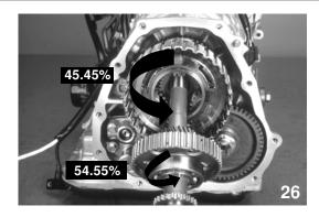
Assuming the friction of the front and rear tires is the same, the power is split 54.55% to the rear and 45.45% to the front.
