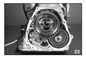
The Pinion Gears are two gears made together. The smaller gear and larger gear have the same number of teeth. The Intermediate Sun Gear drives the smaller Pinion Gear and the larger Pinion Gear.
