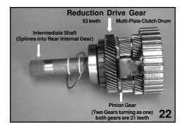
An Intermediate Shaft is splined to the Rear Internal Gear, carrying power to a Sun Gear. The Sun Gear is made onto the end of the Intermediate Shaft. The rotating Sun Gear delivers power to a set of Pinion Gears.
