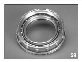
The piston for the MPT Clutch is machined to spline with the MPT Drum. The piston will rotate with the drum.
