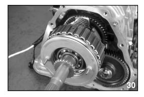
The backside of the piston is made with two locating pins. This prevents the backside of the piston from rotating.
