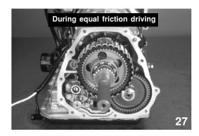
The Front Wheels load the reduction drive and driven gears.
