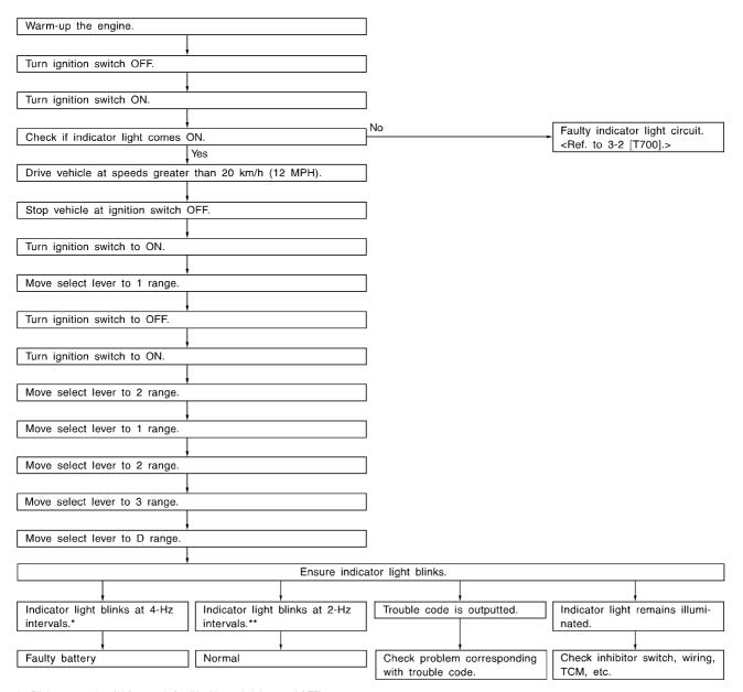
$<sup>^{\</sup>star}$  : Blinks every 0.125 (1/8) seconds (until ignition switch is turned OFF).  $^{\star\star}$  : Blinks every 0.25 (1/4) seconds (until ignition switch is turned OFF).
