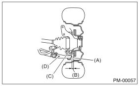
3) Grasp the end of front arm and move it up and down. Relative movement (A) between the housing (D) and front arm (C) boss indicates ball joint (B) may be excessively worn.
