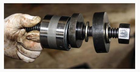
9 Screw the installation bolt through the housing and into the nut on the back of the housing. Secure the nut with a wrench and begin tightening the bolt with an air wrench and socket to seat the bearing. > Make sure to select the correct spacers and adaptors for installing the new bearing.
