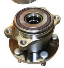
> The Integrated Hub Unit is a sealed component combining the hub, bearing and seals. It is replaced as a whole unit.
