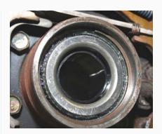
> If the snap ring doesn't properly engage the groove, the bearing isn't fully seated.
