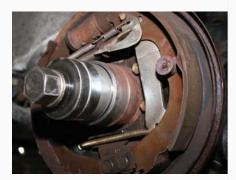
> Tools positioned to install the bearing.
