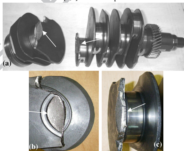
Fig. 4. (a) Failed crankshaft showing the morphology of the surface crack; (b) and (c) the crack initiation sites at crankweb No. 6.
