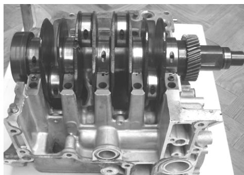
Fig. 2. Boxer crankshaft placed on the bedplate and into the half block's motor.
