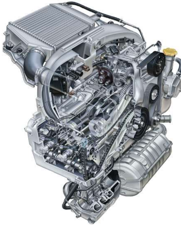
Subaru EE 20 engine, early Euro 4 emissions standard, open-type DPF
