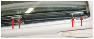
Remove the 8 nuts from the lift bracket; there are 4 on each side.
