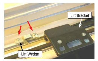
Using the sunroof switch or sunroof wrench, move the lift bracket approximately 4 inches towards the rear of the vehicle. Remove the 2 screws from the lift wedge on each side.
