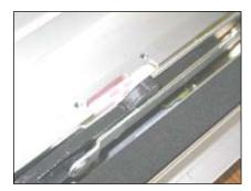
Using the sunroof switch or sunroof wrench, move the lift brackets slightly rearward so that the brackets return to their tracks.
