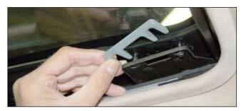
Remove the shims. Pay extra attention to the number of shims in each location. **Note:** At the end of the procedure the shims will need to be reinstalled in their original location to ensure proper glass height adjustment.
