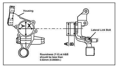
Note: Measure the roundness of the housing where the bearing is installed as follows
