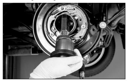
23. Clean and inspect the bearing housing for damage. Use the test outlined below to check for out of roundness condition. Replace bearing housing if out of round.
