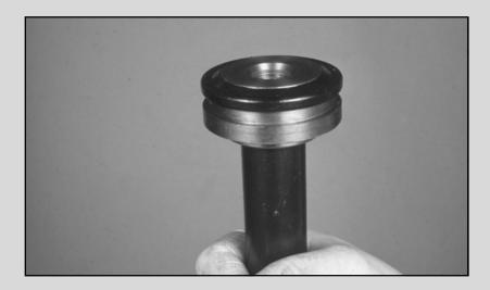
46. Reverse the J 45697-10 on the driver handle J 8092. Place the inner number two seal on the tool and install the seal. The seal is fully installed when the seal is flush with the bearing housing.
