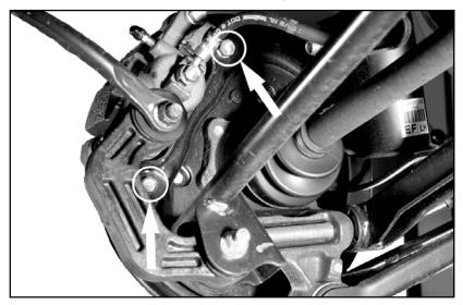
3. Secure the caliper. Place a mark on the hub and rotor so that they can be reassembled the same way they came apart.
