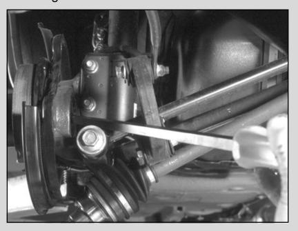
13. Place OTC 311882 over the bearing housing. The groove must face outward.
