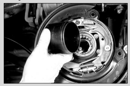
14. Rotate the OTC 311882 as it is installed and make sure it is making full contact with the backing plate.
