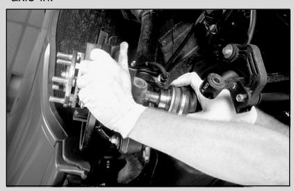
50. Install and torque the lateral link bolt. Use new self locking nut. DO NOT USE IMPACT GUN. Legacy 87-116 ft-lb Impreza and Forester 101 ± 14 ft-lb
