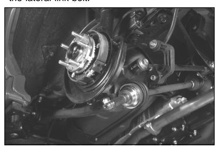
(Inspect the axle for any deep scratches, pitting and damage to the dust shield. Replace if necessary.)
