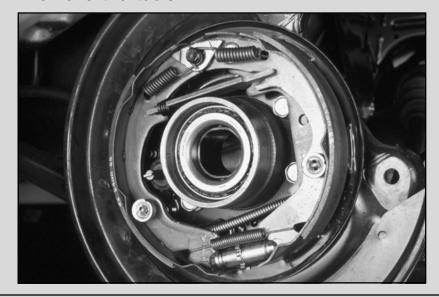
33. Insert the snap ring. If the snap ring will not seat properly the bearing is not fully installed.
