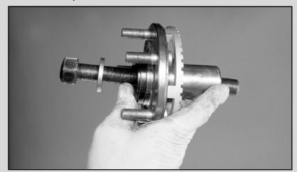
41. Place the J45697-1 with the **smaller** diameter surface facing inward onto the puller bolt after it has been inserted through the bearing housing.
