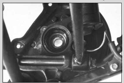
47. Check the rolling resistance of the hub with the supplied torque wrench. The hub should turn smoothly. (Starting force should be 7 to 17 inch pounds.)
