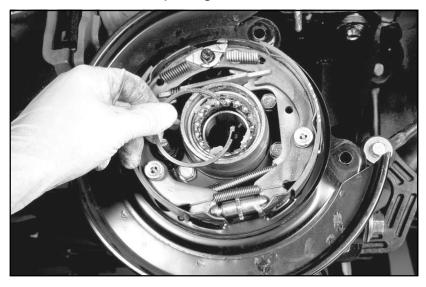
12. Remove the inner seals from the bearing housing.
