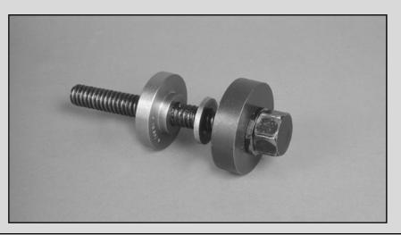
27. The J45697-1 larger diameter surface will face the wheel bearing housing on the inner side after the puller bolt has been inserted into the bearing housing.
