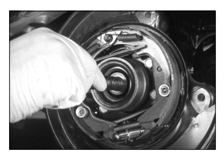
37. Prepare the hub for installation. Remove the old outer seal from the hub.
