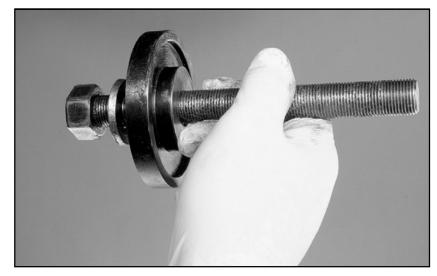
18. The OTC 311887 with washer and nut will be placed onto the opposite end of the puller bolt after it has been inserted into the bearing housing. If the wrong side of OTC 311887 is placed against the bearing the tool will become jammed into the inner race.
