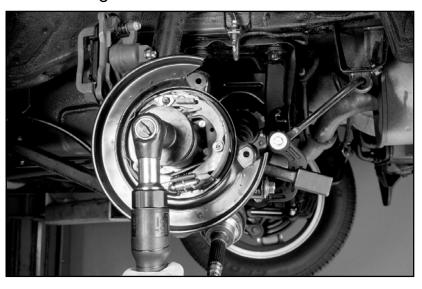
22. Remove the bearing and tools from the outside of the bearing housing.
