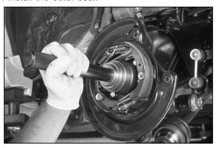
36. Remove all tools from the puller bolt. Push out the bearing stay from the center of the installed bearing using the head of the bolt.
