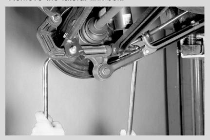
7. Push the bearing housing outward and slide the axle out.
