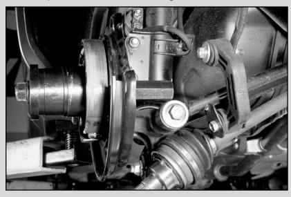
20. Secure a wrench on the nut located on the backside of the bearing housing. Using a breaker bar begin tightening the puller bolt.
