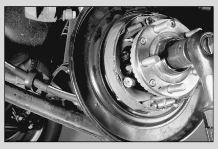
44. Check the installed depth of the hub with the following procedure. Measure through the provided slot on J45697-1. (Remove the washer if necessary and reinstall nut) Using an appropriate depth gauge measure from the top of J-45697-1 to the top flat edge of the wheel bearing. This will represent "A".
