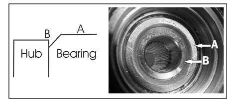
45. Thread seal installer J 45697-10 onto driver handle J 8092 with the pictured surface facing outward. Place the inner number one seal on the tool and install the seal. The tool will make contact with the bearing housing when the seal is fully installed.
