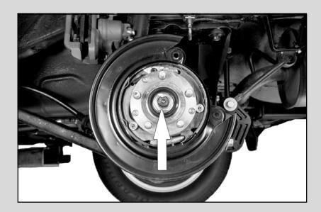
6. Remove the lateral link bolt.
