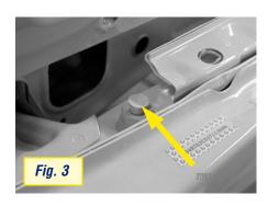
If the bumper plugs are not removed, this may cause difficulty in properly installing the trailer hitch bolt. It may be a good idea, when initially threading the bolt into the bumper beam weld nut, to start it by hand. This will avoid cross-threading the bolt. For proper installation instructions, please download the information from http://www.subarunet.com
