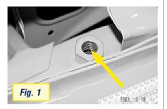
The bumper beam plugs are installed at the factory to prevent the inside on the threads from being painted (see Fig. 2 and 3).
