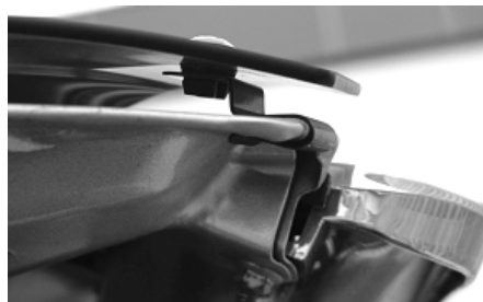
3M Adhesive Strips included in New Deflector Kit to protect paint surfaces from clips.
