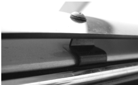
Installation of Center Clip on New Deflector requires R&R of Grille.
