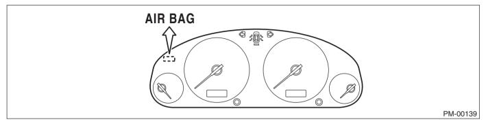
2) Turn the ignition switch ON, and connect the airbag diagnosis terminal of the service connector (located below lower cover) to the ground terminal.
